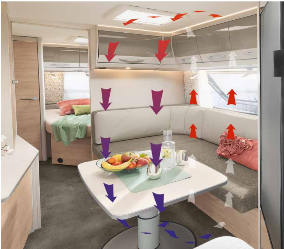
AirPlus ventilates the overhead lockers and thus prevents the formation of condensation
