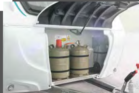
Gas bottle locker for 2 x 11 kg bottles with base made of rot-proof, sturdy aluminium chequer plate
